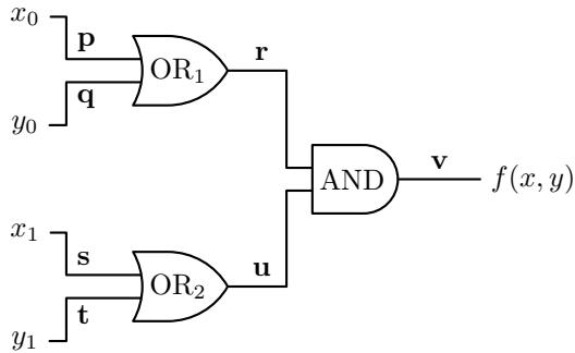
The above figure represents the circuit of  $f$ .  $A$ 's input bits ( $x_0$  and  $x_1$ ) are on the input wires  $\mathbf{p}$  and  $\mathbf{s}$ .  $B$ 's input bits ( $y_0$  and  $y_1$ ) are on the input wires  $\mathbf{q}$  and  $\mathbf{t}$ .
